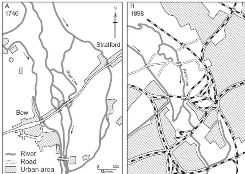
Figure 2: The anastomosing course of the River Lea in 1746 and 1898 showing the encroachment of urban, industrial and railway development onto the floodplain (the development of railways is illustrated by the hatched black and white lines) 14 .
