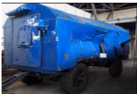
Figure 19: Damage caused to the containers and trailers
