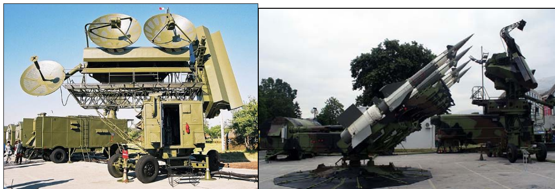
Figure 1: Complete SA-2 Fan Song 3 and complete SA-3 Pechora system with Low Blow radar
