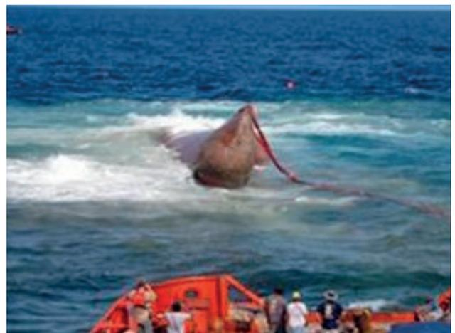
*The container ship Angeln is refloated with compressed air.*
